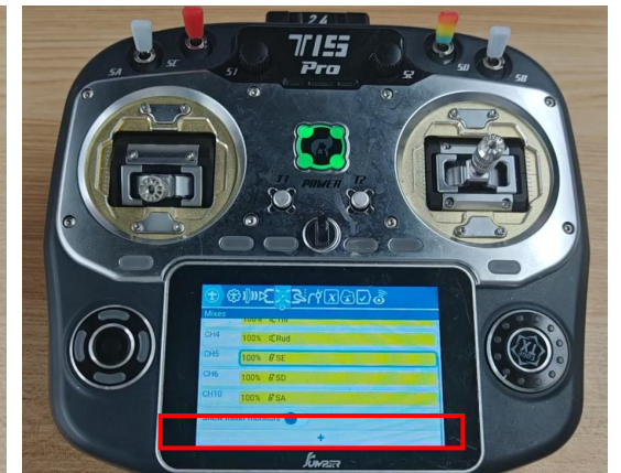
8. The lock switch (SA) is displayed in the list, channel setup completed successfully.
