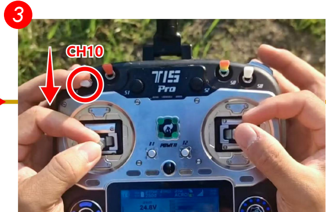
3 Push the CH10 switch down to enter hard lock mode
