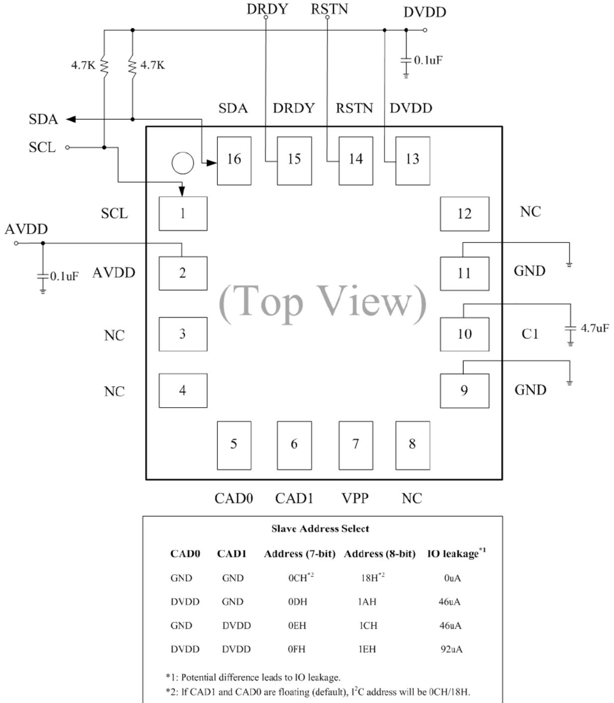
Figure 2. Application Circuit
