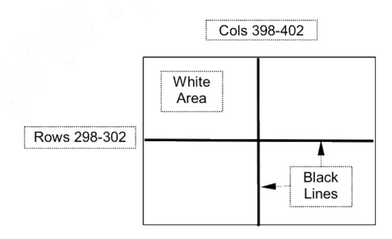
TEST PATTERN FOR IMAGE STICKING TEST
