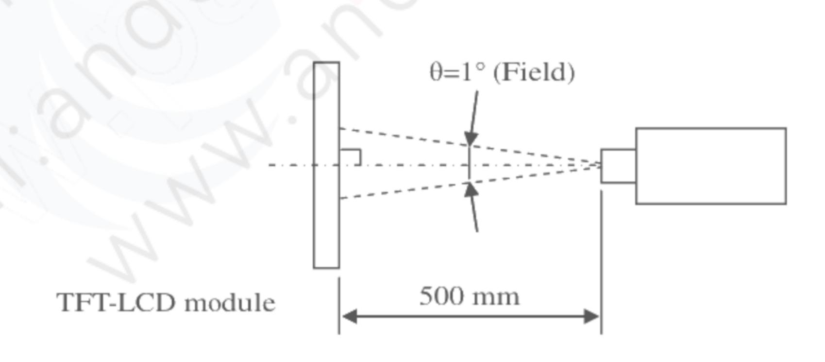
The luminance is measured according to FLAT PANEL DISPLAY MEASUREMENTS STANDARD (VESA Standard).
