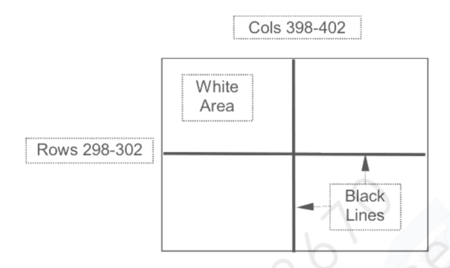
TEST PATTERN FOR IMAGE STICKING TEST
