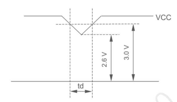
\*2) VCC = +3.3 V , f<sub>H</sub>=48.36 kHz, f<sub>V</sub>=60 Hz, f<sub>CLK</sub>=65 MHz Display image at typical power supply current value is 256-gray-bar pattern (8 bit), 768 line mode.
