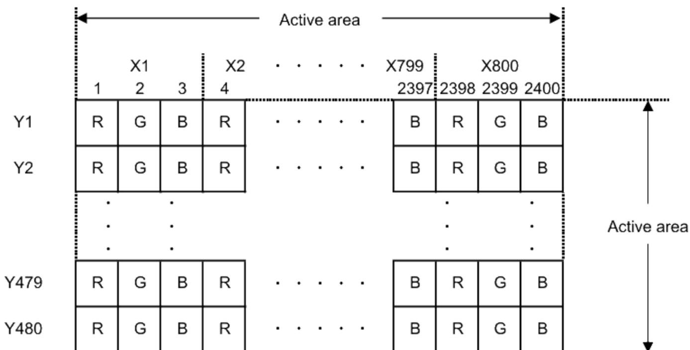
Dot arrangement (FPC cable placed down side)
