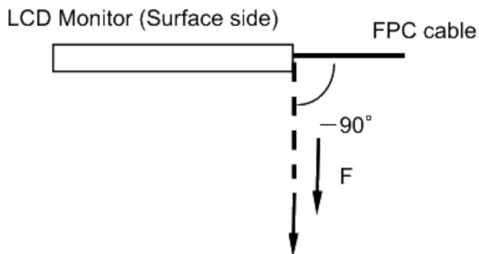
Bend Test Method for FPC cable
