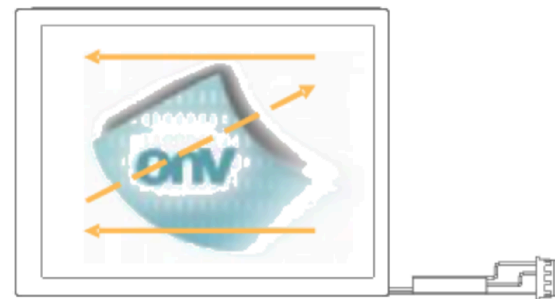
Fig. 2 Reverse scan (Pin4, DPS = High)
