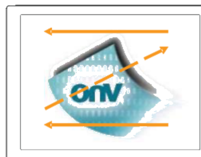
Fig. 2 Reverse scan (Pin19, RSV = High or VDD)
