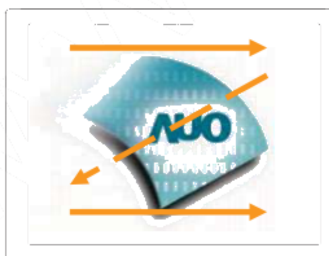
Fig. 1 Normal scan (Pin19, REVERSE = Low or NC)
