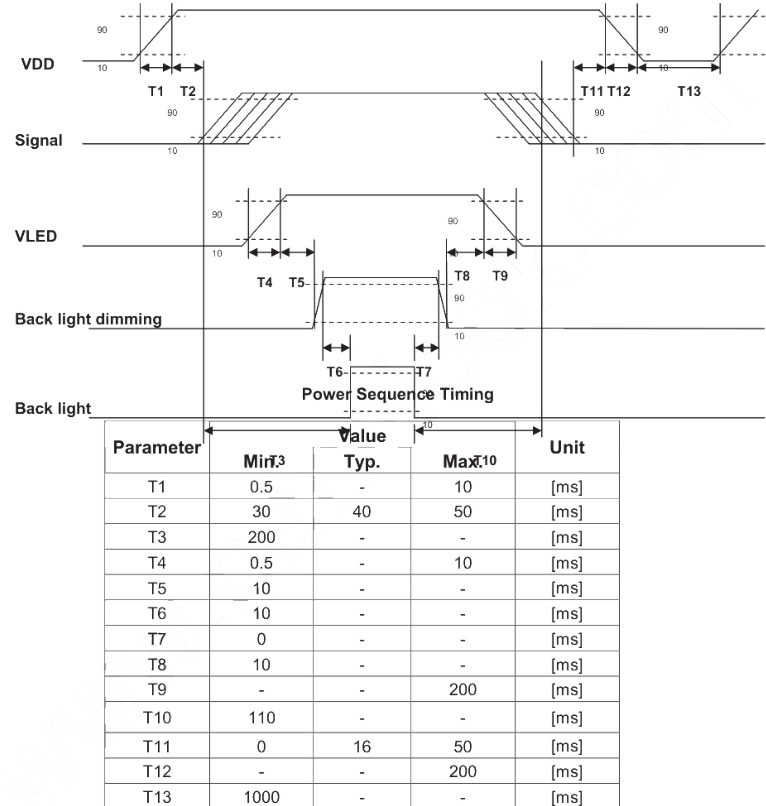
The above on/off sequence should be applied to avoid abnormal function in the display. Please make sure to turn off the power when you plug the cable into the input connector or pull the cable out of the connector.
