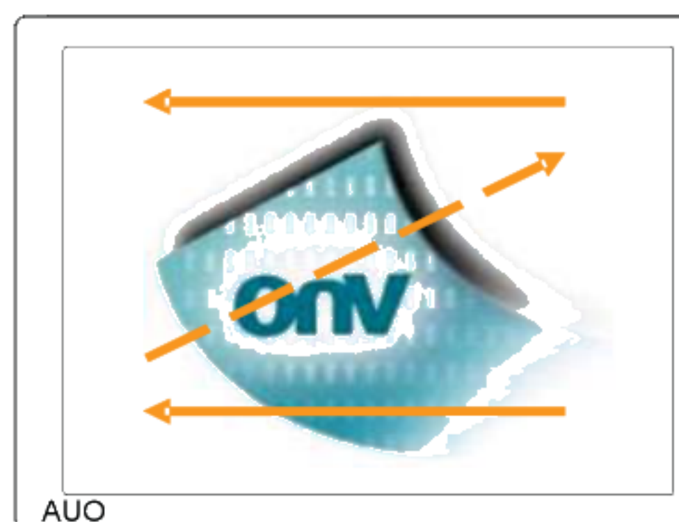
Fig. 2 Reverse scan (Pin4, REV = High)
