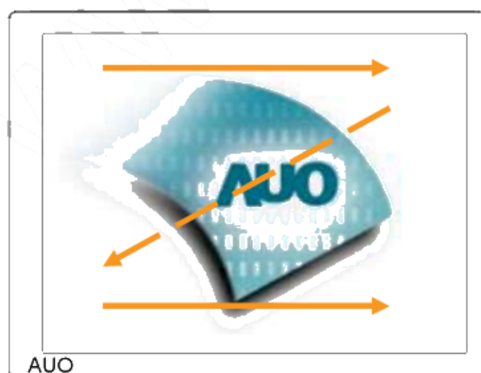
Fig. 1 Normal scan (Pin4, REV = Low or NC)
