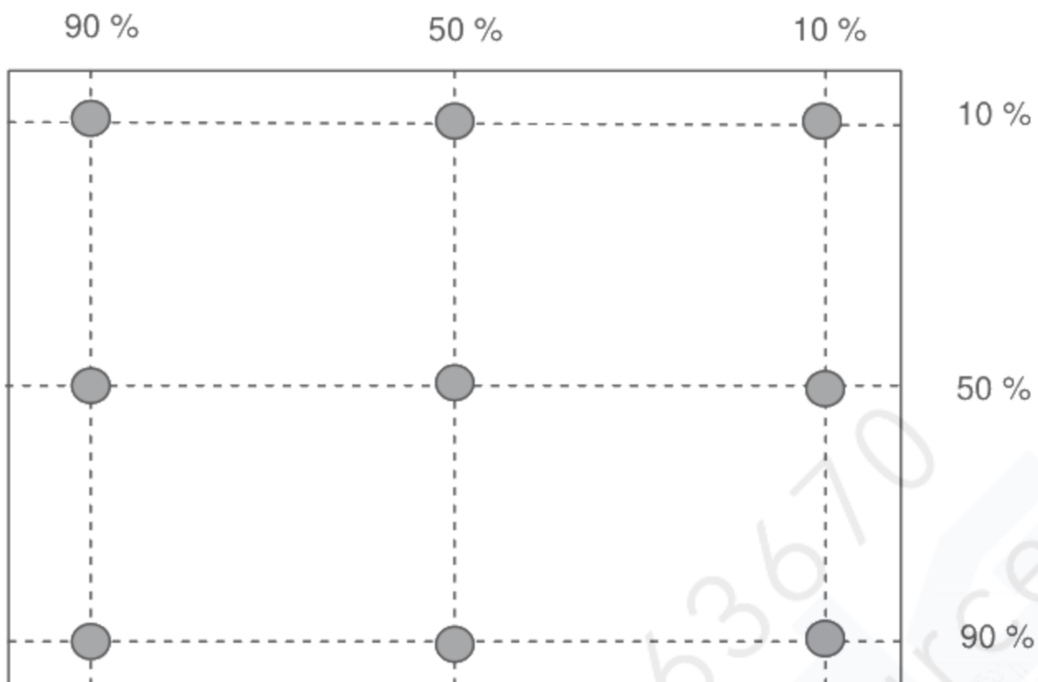
Note 3: The luminance uniformity of 9 points is defined by dividing the minimum luminance values by the maximum test point luminance
