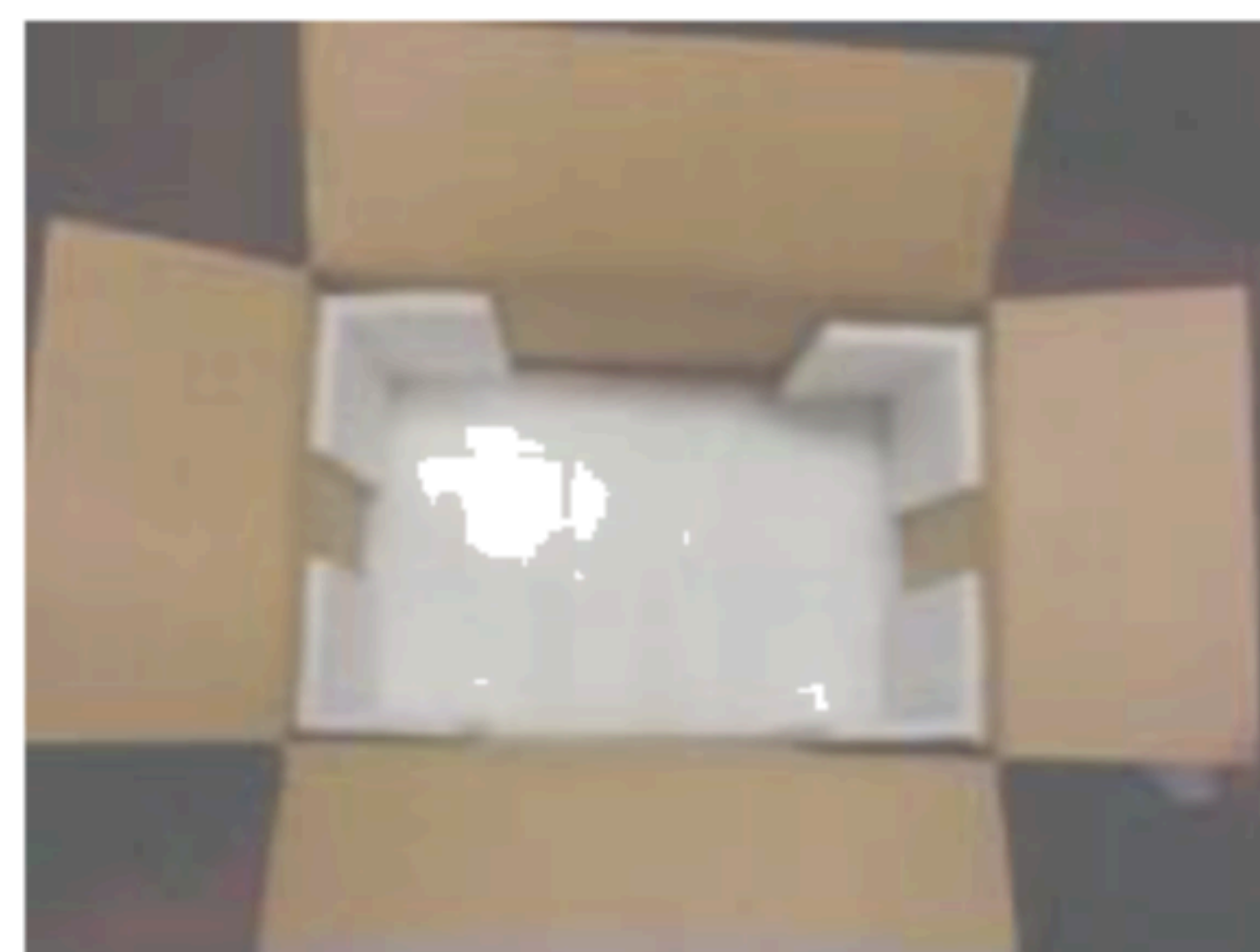
8 - Placing EPE into carton
