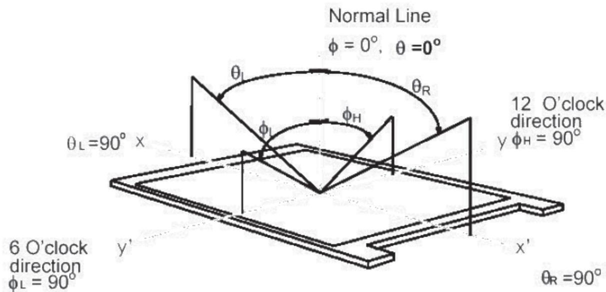
Crosstalk above for viewing angle under 3D mode is defined as below:
