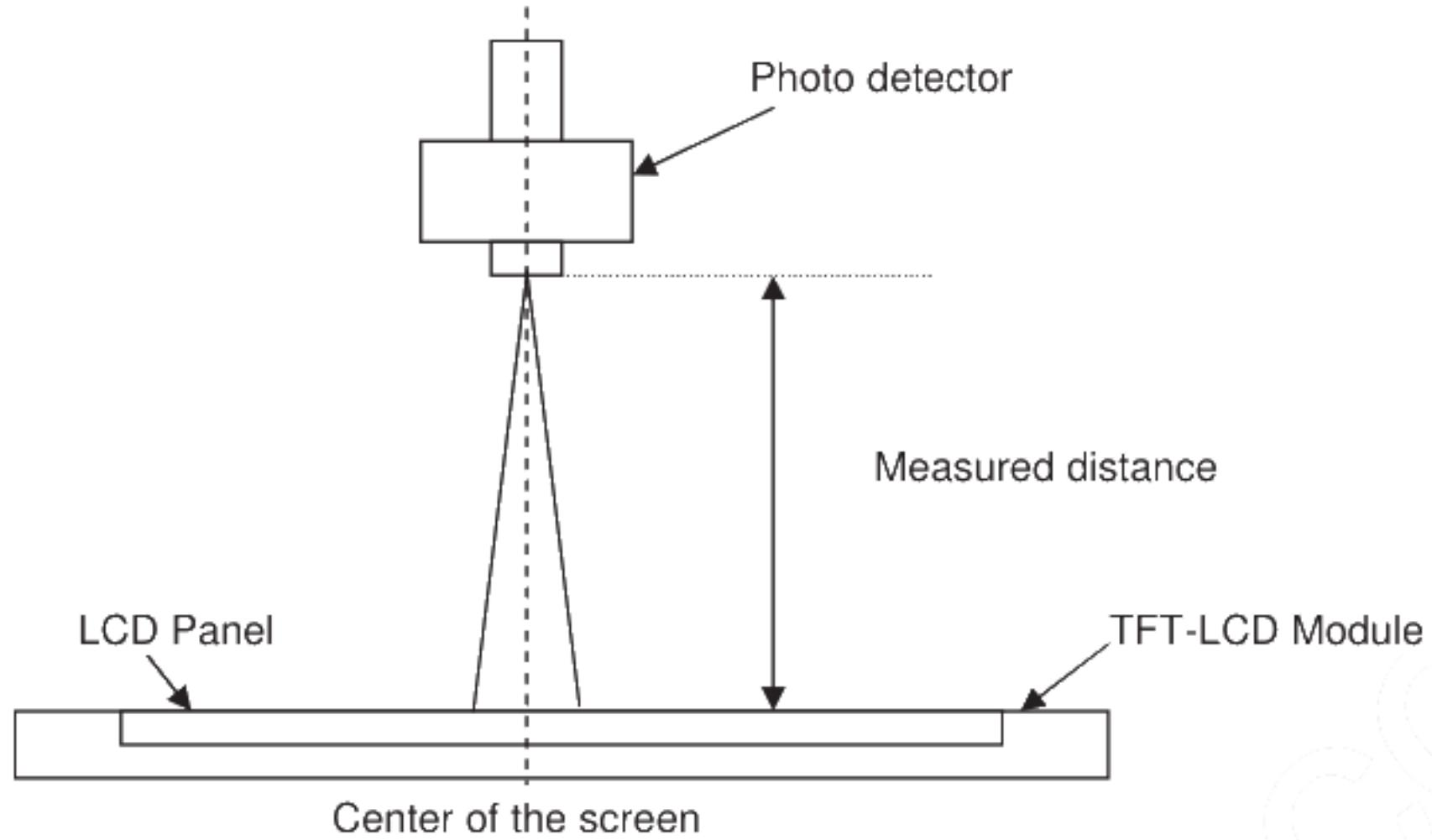
**Note 2: Definition of viewing angle measured by ELDIM (EZContrast 88)**
