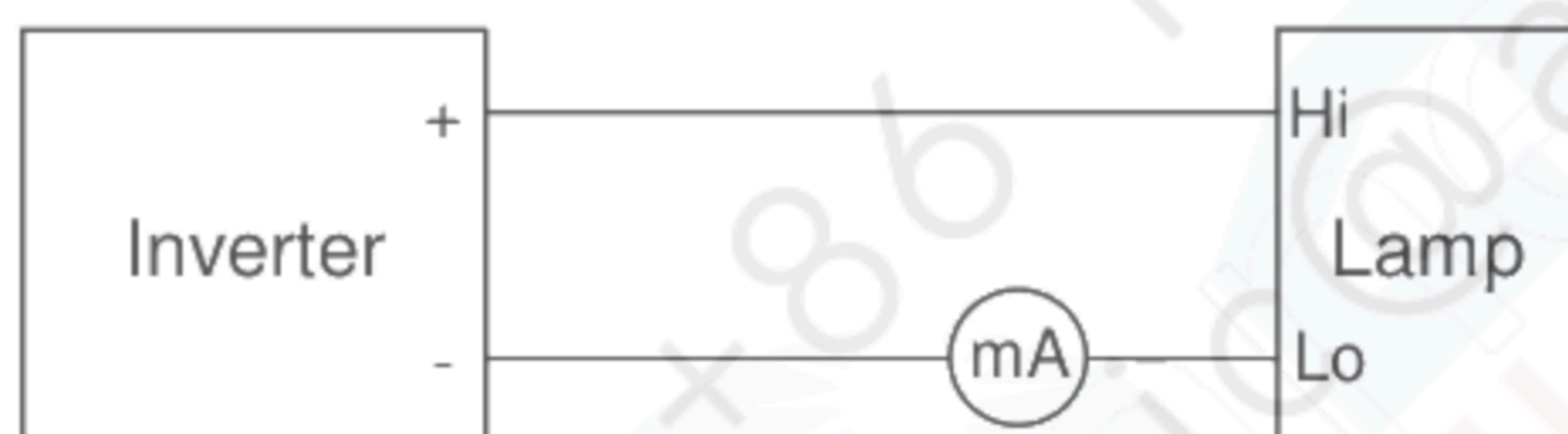
(Figure. 1: Measurement of return current)
