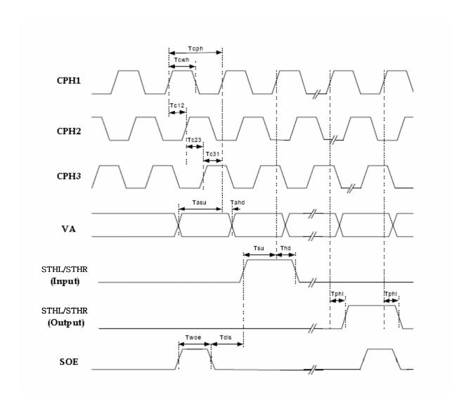
• Remark: The sample-and-hold circuits are switched and the outputs are started with new data at the rising edge of SOE.
