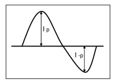
\* Asymmetry rate:  $\left( \mid_{p} - \mid_{-p} \mid \right) / \mid_{rms} * 100\%$  • Distortion rate:  $\mid_{p} \left( \text{or } \mid_{-p} \right) / \mid_{rms}$
