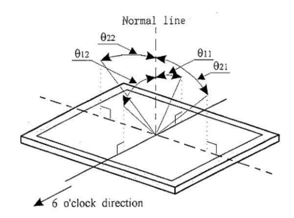
The best viewing angle of this module is slightly leaned to  $\,6\,$  o'clock from normal line. In the field where  $\,\theta_{12}\,$  exceeds this angle, gray-scale is reversed partially. The gray-scale in the field of 12 o'clock direction is brighter than that of  $\,6\,$  o'clock direction and isn't reversed.
