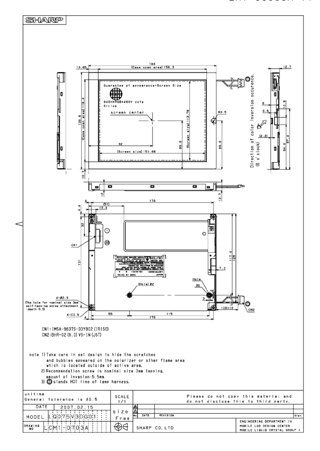
Fig. 1 DIMENSIONS OF THE MODULE
