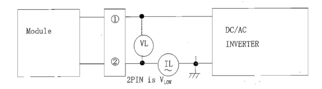
[Note6-8] The voltage at the output of inverter circuitry.
