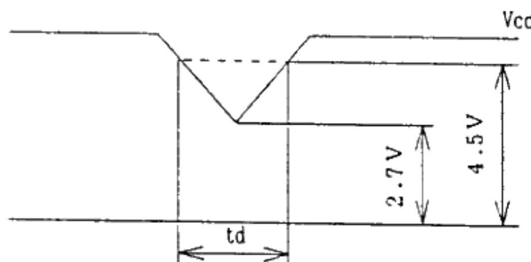
V<sub>CC</sub>-dip conditions should also follow the V<sub>CC</sub>-turn-on conditions.
