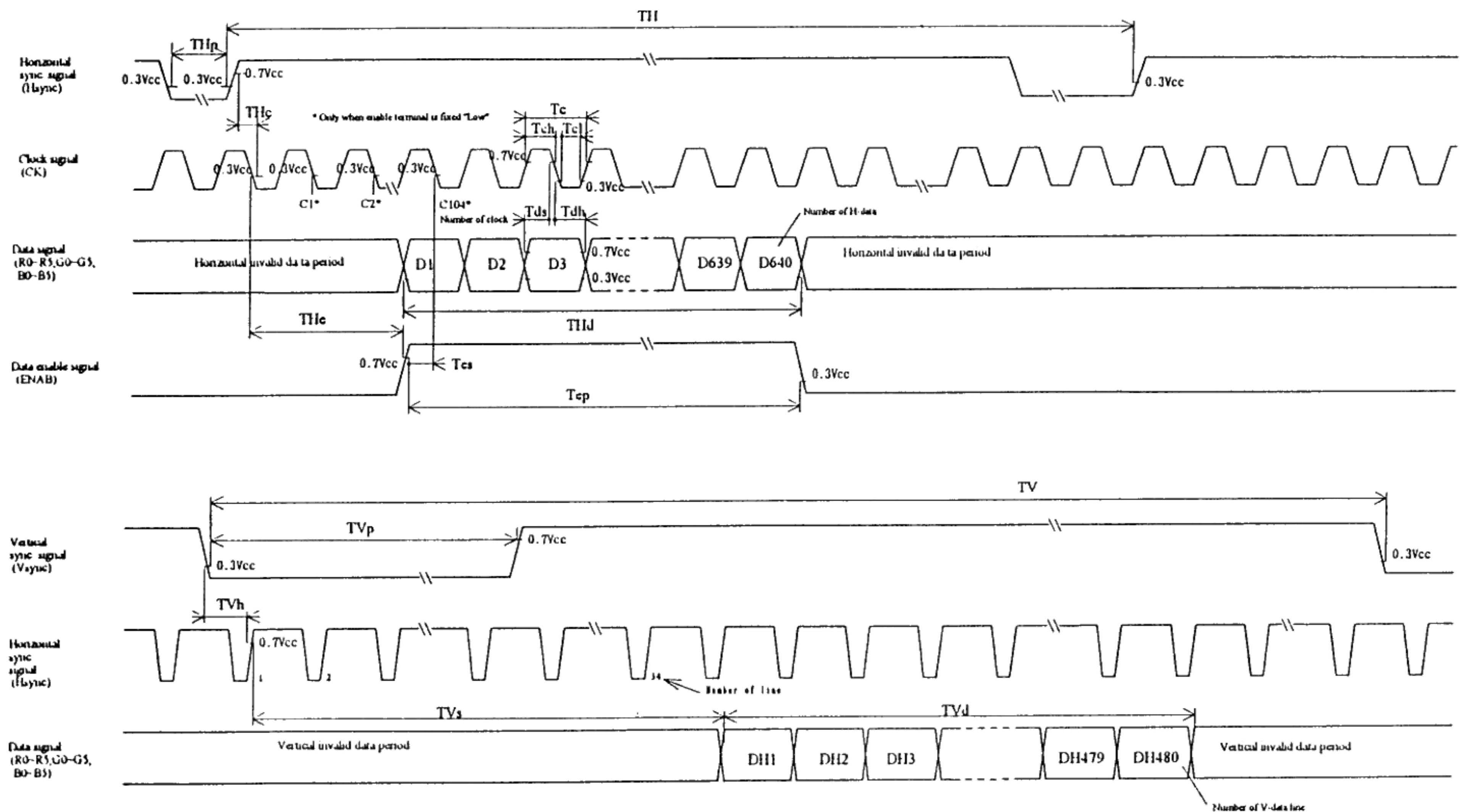
Fig 2-1 Input signal waveforms (480 line mode)
