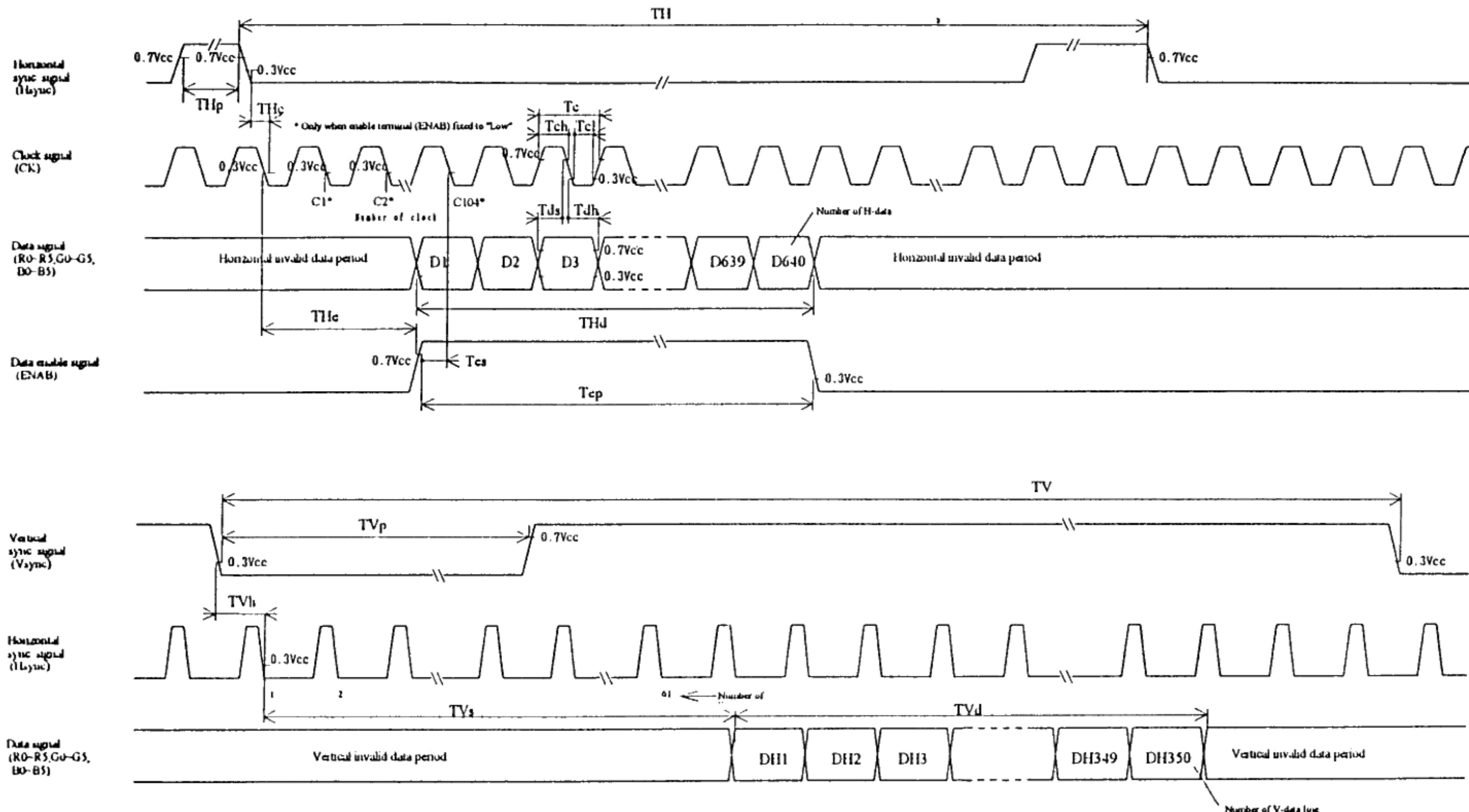
Fig.2-3 Input signal waveforms (350 line mode)
