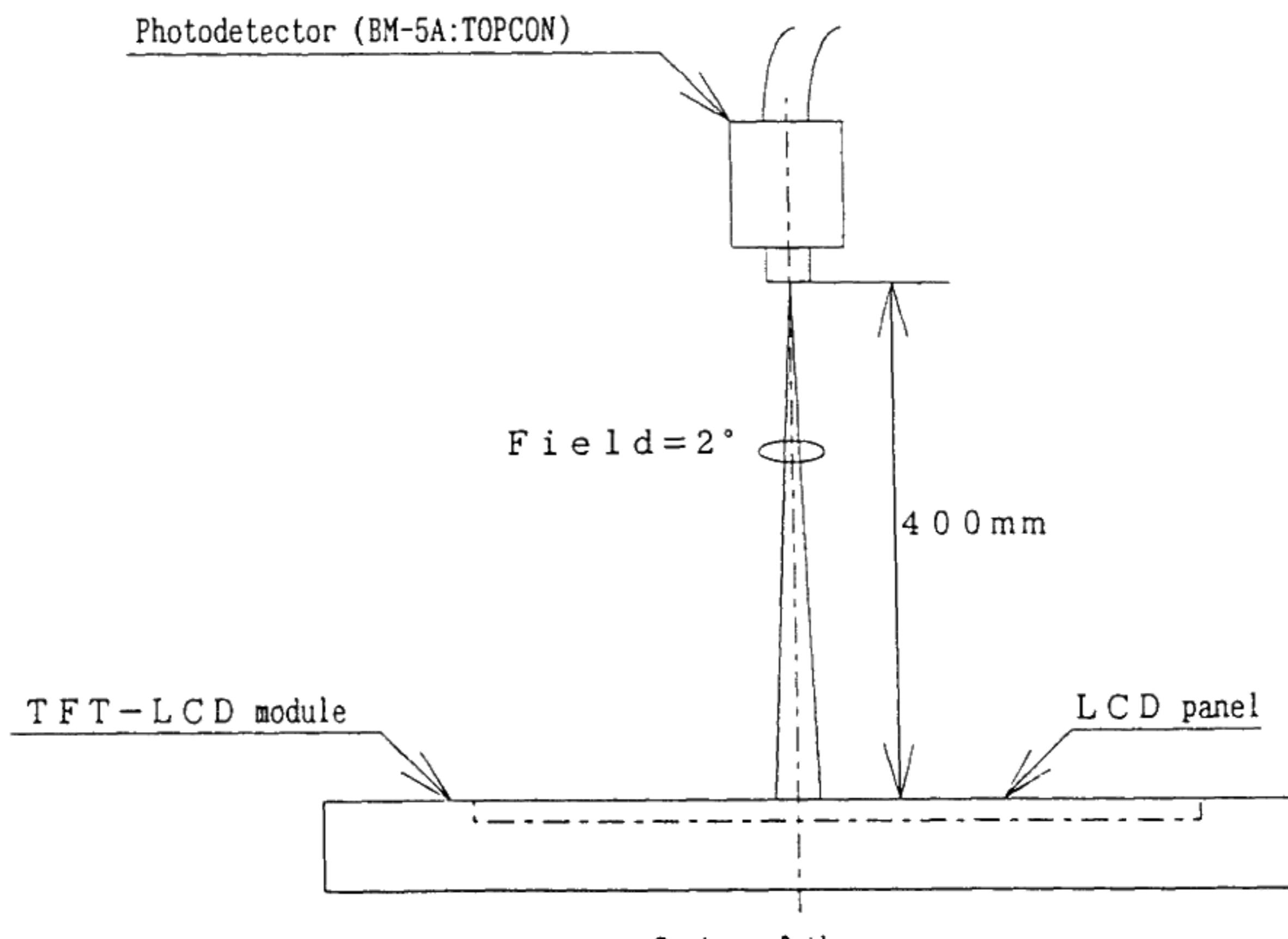
Fig.3 Optical characteristics measurement method
