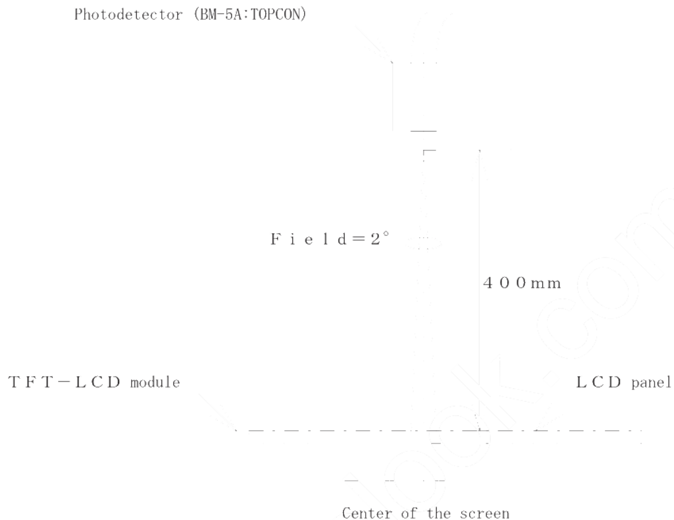
Fig.3 Optical characteristics measurement method
