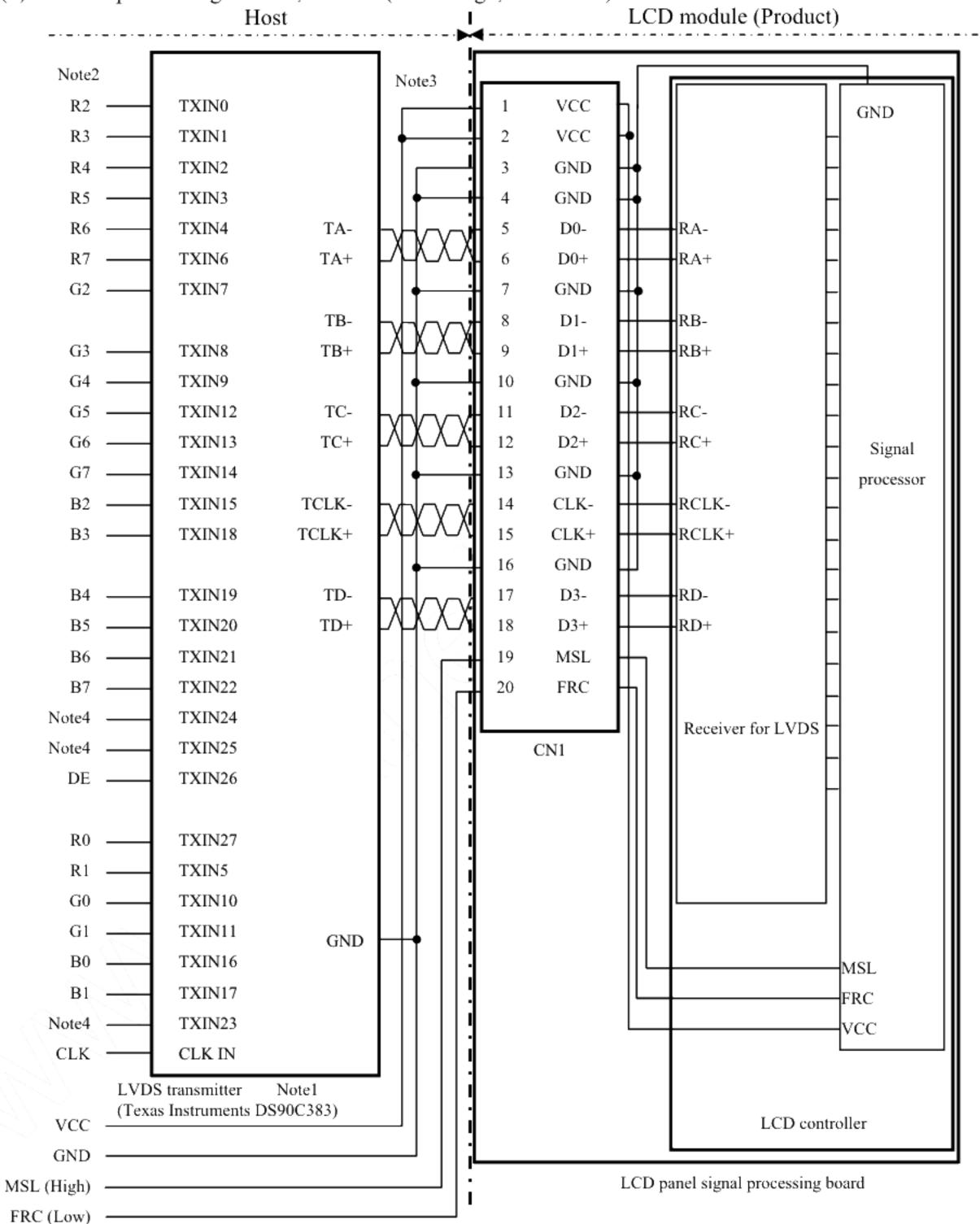
Note1: Recommended transmitter. See the data sheet for DS90C383 (Texas Instruments).
