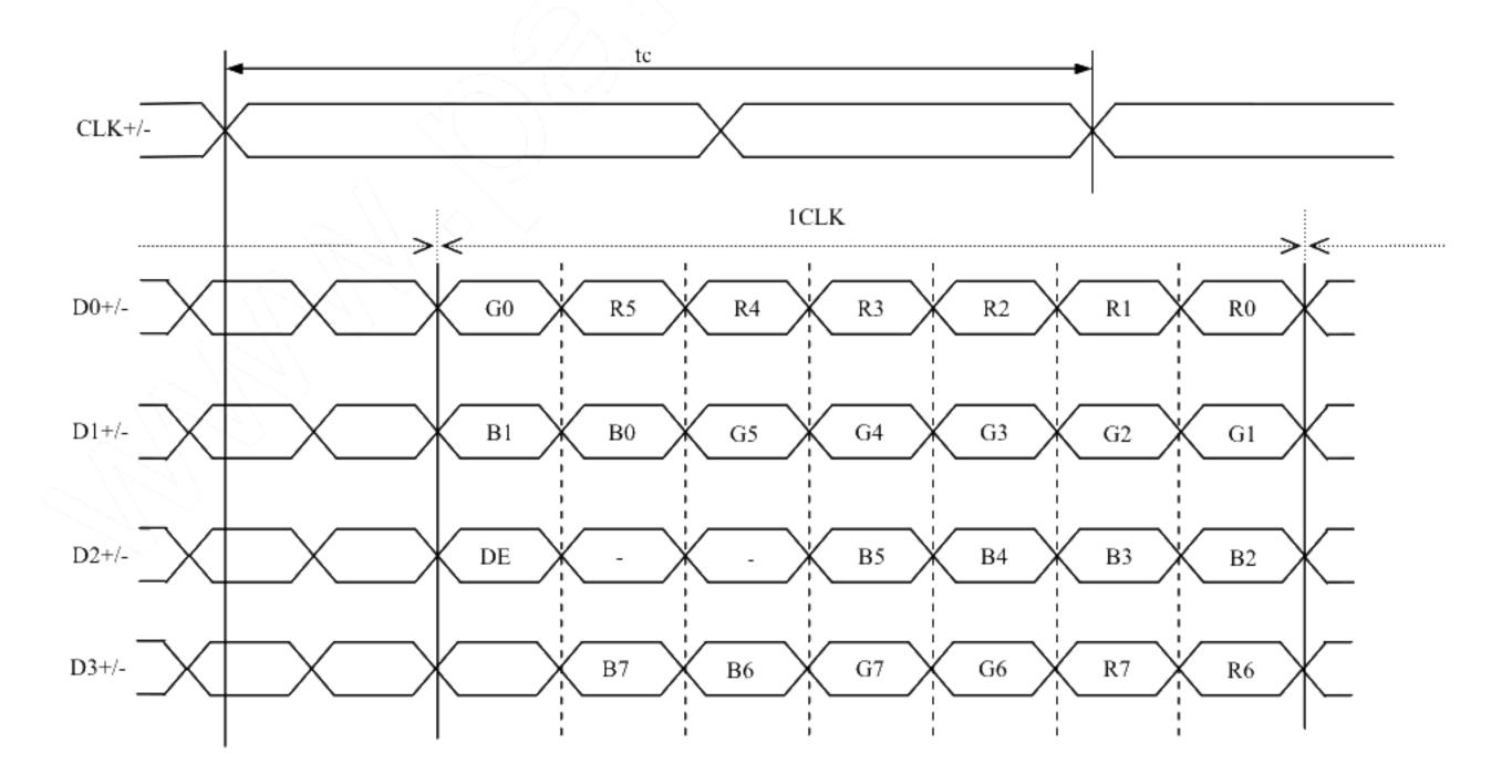
(3) LVDS Input data signal: 6bit (MSL: High, FRC: High or Open)
