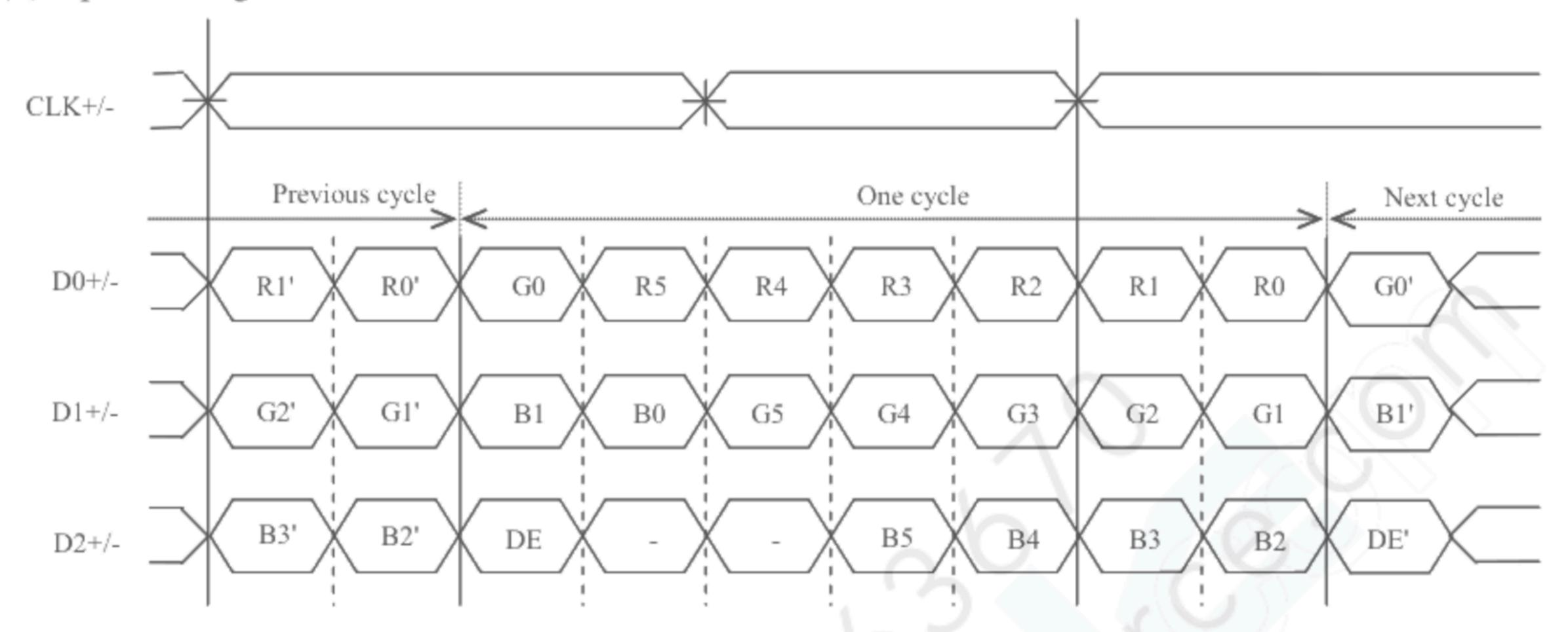
Note1: LSB (Least Significant Bit) - R0, G0, B0 MSB (Most Significant Bit) - R5, G5, B5
