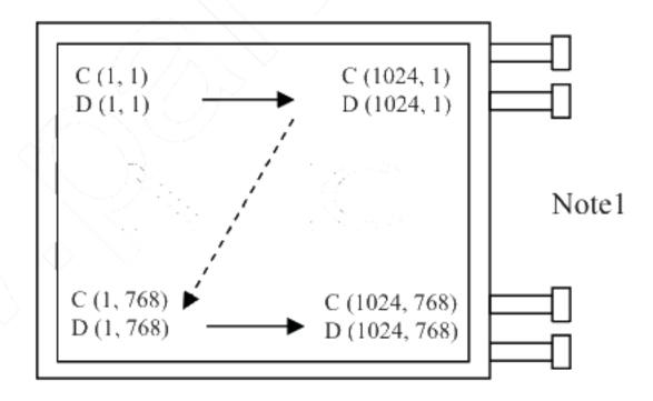
Note1: Meaning of C (X, Y) and D (X, Y)
