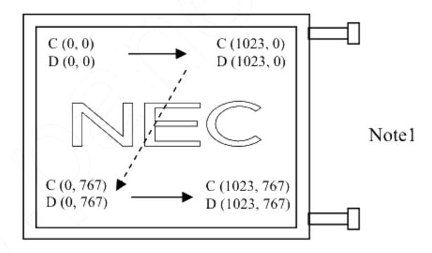
Note1: Meaning of C (X, Y) and D (X, Y)
