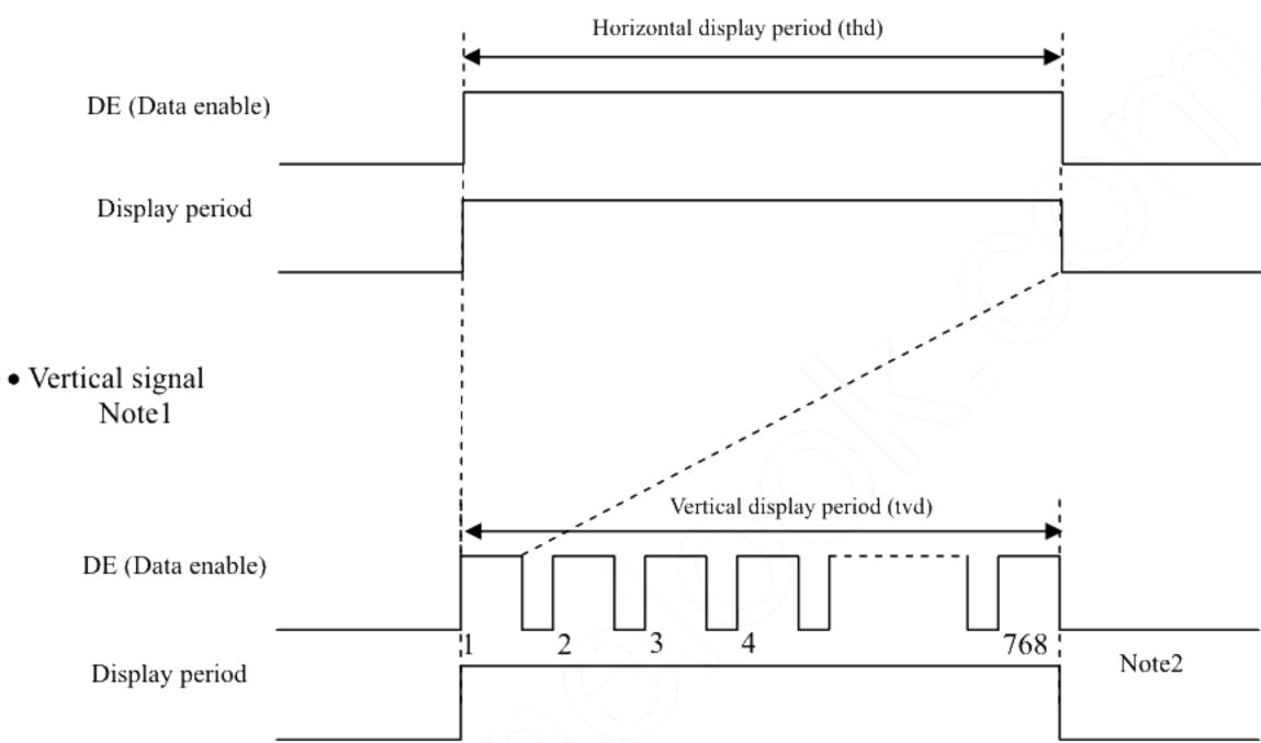
Note1: This diagram indicates virtual signal for set up to timing. Note2: See "4.9.3 Input signal timing chart" for the pulse number.
