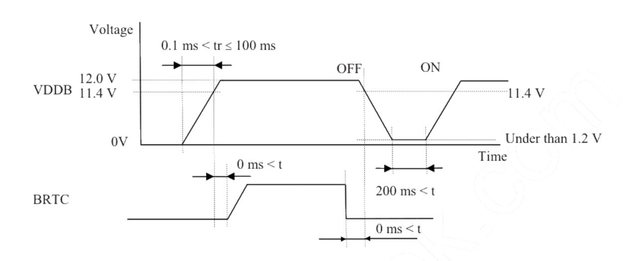
Note1: The backlight should be turned on within the valid period of LVDS signals, in order to avoid unstable data display.
