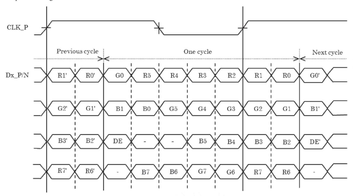
Note1: LSB (Least Significant Bit) – R0, G0, B0 MSB (Most Significant Bit) – R7, G7, B7
