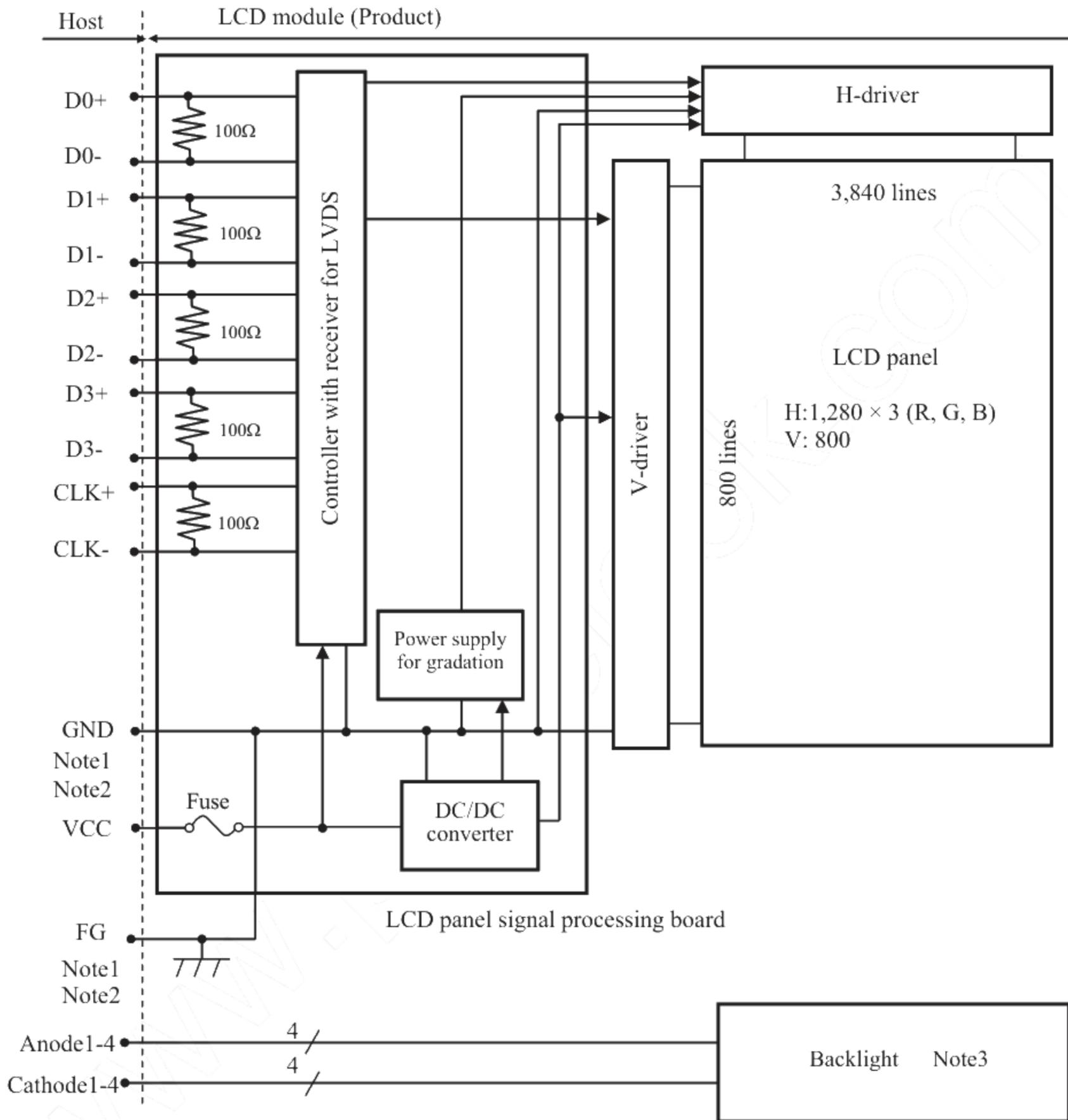
Note1: Relation between GND (Signal ground) and FG (Frame ground) in the LCD module is as follows.
