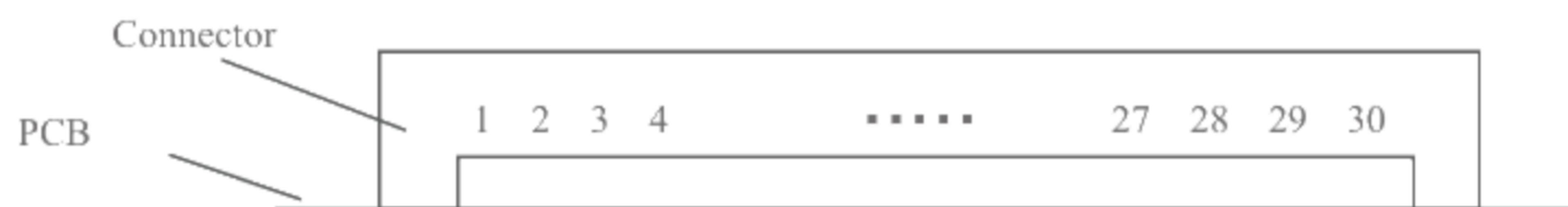
Note1: Twist pair wires with  $100\Omega$  (Characteristic impedance) should be used between LCD panel signal processing board and LVDS transmitter.
