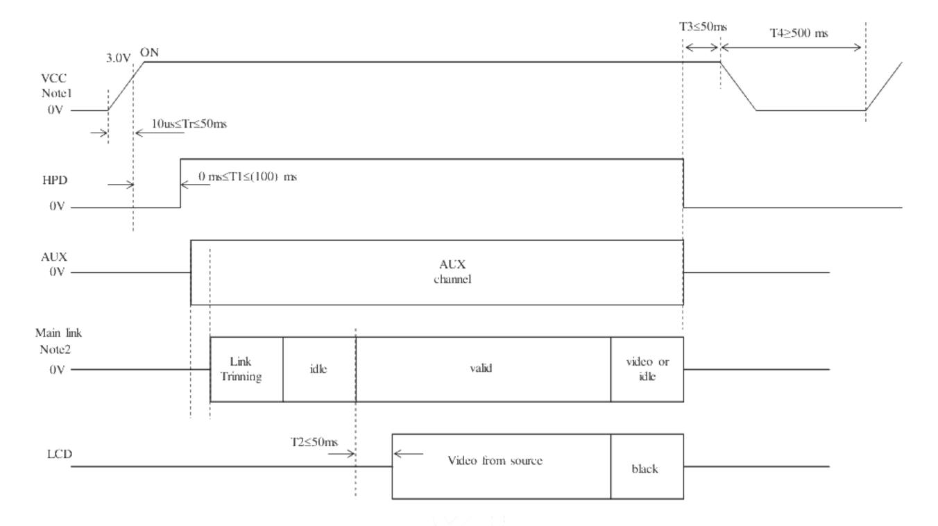
Note1: If there is a voltage variation (voltage drop) at the rising edge of VCC below 3.0V, there is a possibility that a product does not work due to a protection circuit.
