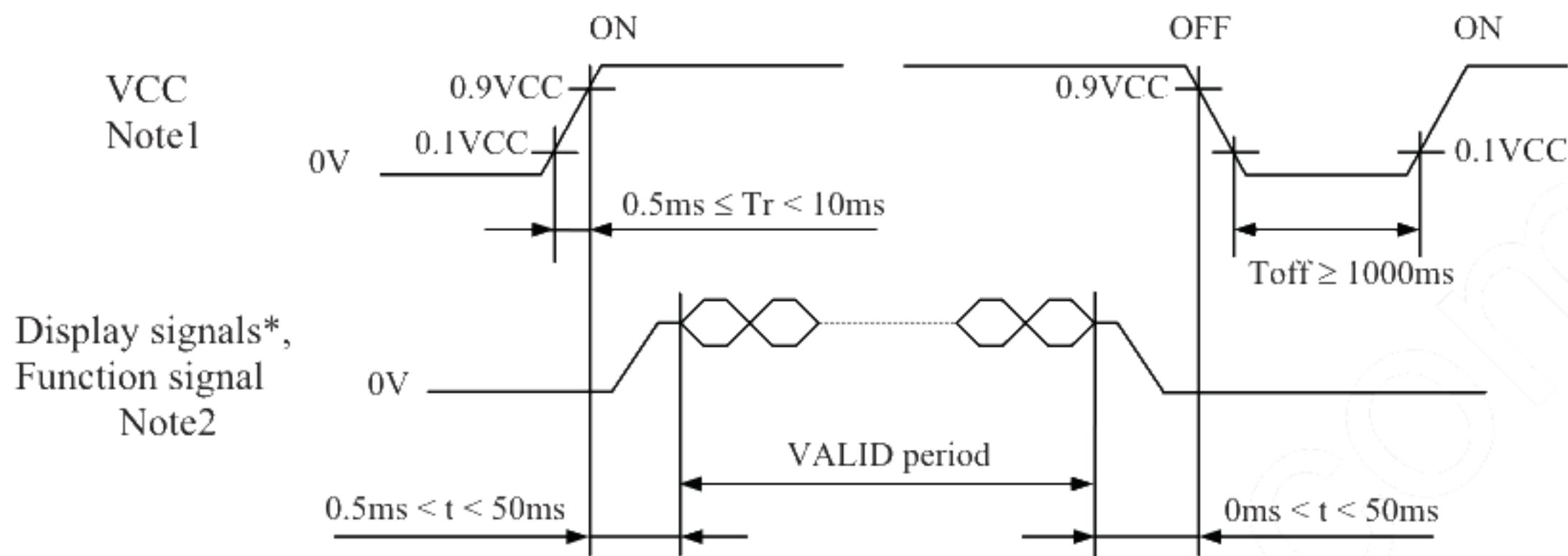
\* These signals should be measured at the terminal of  $100\Omega$  resistance.
