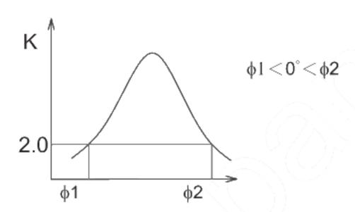
Contrast ratio K vs viewing angle \$\phi\$
