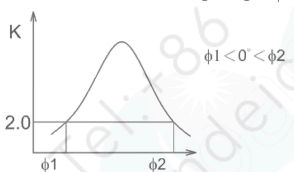
Contrast ratio K vs viewing angle o
