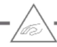
\* Do not shock and press the LCD panel and the backlight! There is a danger of breaking, because they are made of glass. (Shock: Equal to or no greater than 294m/s<sup>2</sup> and equal to or no greater than 11ms, Pressure: Equal to or no greater than 19.6 N (\$\phi16mm jig))
